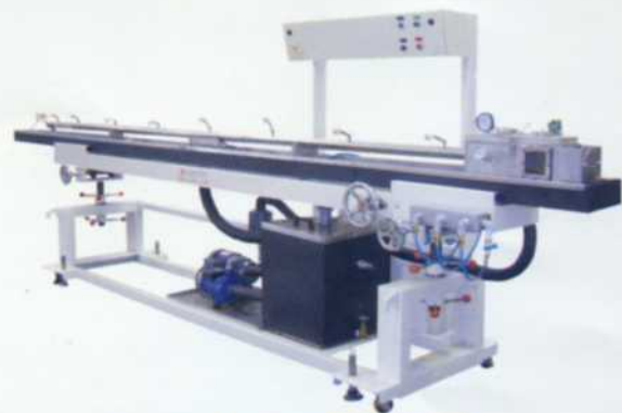
Vacuum Water Tank
